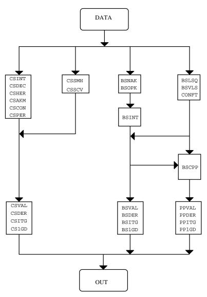
Figure 3-2 Interrelation of the Spline Routines
