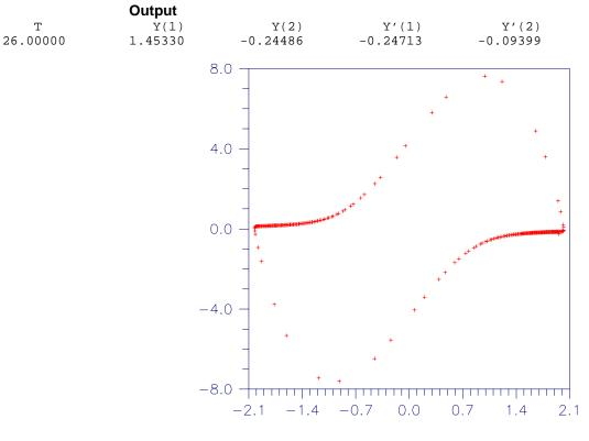
Figure 5-1 Van der Pol Cycle, (u(t), u'(t)),  $\mu = 5$ .
