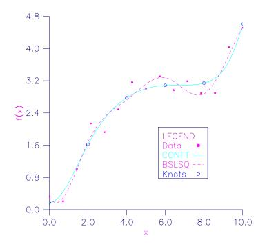
Figure 3-8 CONFT vs. BSLSQ Forcing Monotonicity
