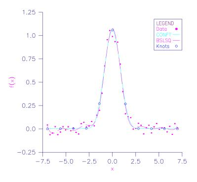
Figure 3-9 CONFT vs. BSLSQ Approximating  $1/(1 + x^4)$
