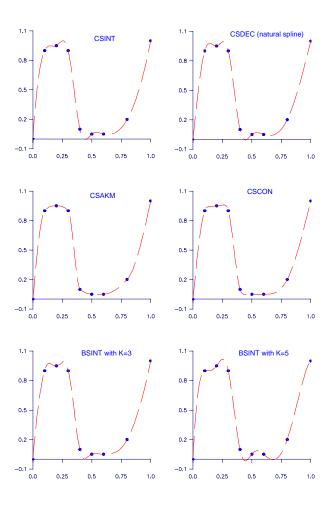
Figure 3-1 Spline Interpolants of the Same Data
